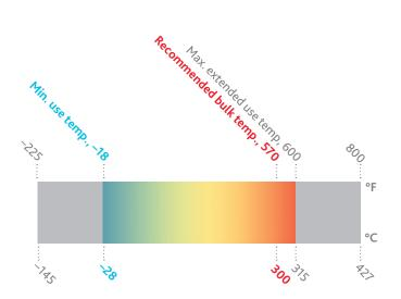
Eastman Therminol® 55 heat transfer fluid is a unique, synthetic fluid designed to provide reliable, consistent heat transfer performance over a long life at recommended bulk temperatures up to 300°C (570°F).
