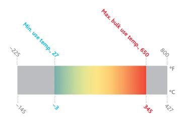
Eastman Therminol<sup>®</sup> 66 heat transfer fluid offers outstanding high-temperature performance to 345°C (650°F), including excellent thermal stability and low vapor pressure. These properties result in reliable, consistent performance of heat transfer systems over long periods of time. Therminol 66 performance is proven through many years of industrial experience under a wide range of operating conditions. No heat transfer fluid material in the world has had more success than Therminol 66.
