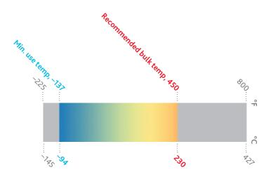
Eastman Therminol® D-12 heat transfer fluid is a liquid phase heat transfer fluid specially developed for process cooling combined with moderate heating cycles using a single fluid in place of the traditional dual steam/brine or steam/glycol systems.
