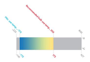
Eastman Therminol® VLT heat transfer fluid is a uniquely formulated liquid-phase fluid with excellent heat transfer and fluid properties for use in extremely low-temperature applications. This fluid offers exceptional low-temperature pumpability and thermal stability and is ideally suited for single-fluid heating and cooling systems between –115°C (–175°F) and 175°C (350°F).
