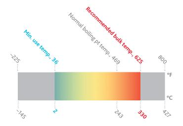
Eastman Therminol® VP-3 liquid/vapor phase heat transfer fluid was specially developed to allow vapor phase heat transfer at lower temperatures than are practical with traditional diphenyl oxide/biphenyl constituted fluids.
