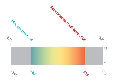
Eastman Therminol® XP heat transfer fluid is an extremely pure white mineral oil which provides low toxicity and reliable heat transfer at moderate temperatures. When operating temperatures prohibit the use of steam or steam is not readily available, Therminol XP can provide safe and efficient operation in heat transfer systems.
